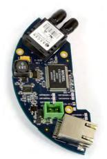
The ComNet<sup>™</sup> series of Ethernet media converters are designed to transmit and receive 10/100 Mbps data over one or two multimode or single mode optical fibers. They are designed to be mounted within an Aigis dome and provide optical Ethernet connectivity.
