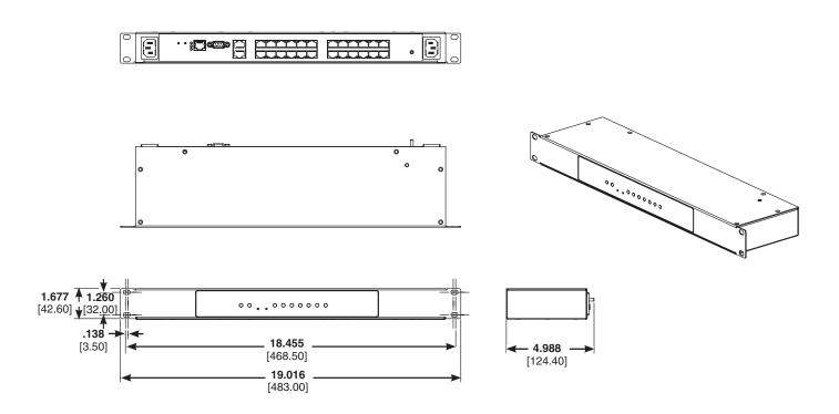
Dimensions are in inches. [Dimensions in brackets are metric].
