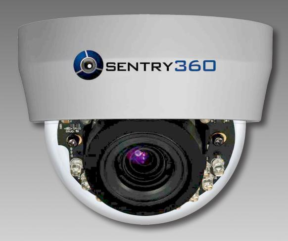
The IS-DM200 camera is a Quad-streaming, H.264 & MJPEG encoding, 2.0 Megapixel resolution, IP-ad-dressable, network camera. It is designed to deliver full-motion, high-definition, progressive scan digital video across local area networks. The IS-DM200 features a 1/2.8" CMOS sensor, Power over Ethernet, 21 IR LED, Audio-In and Audio-Out. The IS-DM200 is a cost-effective, high-level, megapixel network camera.
