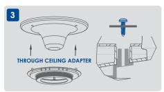
Attach the 'Through Ceiling Adapter' to the antenna and fasten it as outline in figure 3 using the three self-taper screws and washer provided with the mounting kit.
