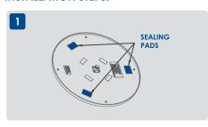
Remove the three 'through ceiling hole' sealing pads from the bottom plate as outlined in figure 1.
