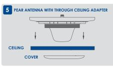
Put the antenna with attached 'Through Ceiling Adapter' through the hole in the ceiling and fasten the antenna to the ceiling with the provided 'Through Ceiling Cover'.
