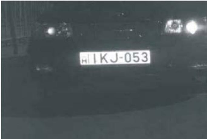
Figure 1. License plate detected at night with IR illuminator
