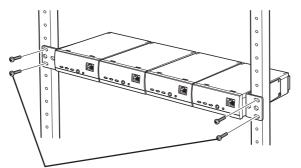
Rack mounting screw (customer-provided, nominal diameter 5 mm [3/16 inches] tapping)
