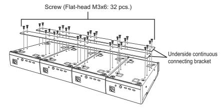
2. Secure the BY-HCA10A mounting brackets to both sides of the connected center adaptors with the screws included with the BY-HCA10A. (Recommended torque 0.4-1.0 N·m {4.1-10.2 kgf·cm})
