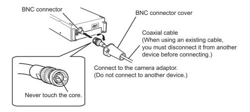
5. Secure the BNC connector cover with the included screw to the center adaptor. (Recommended torque 0.4-0.8 N·m {4.1-8.2 kgf·cm})
