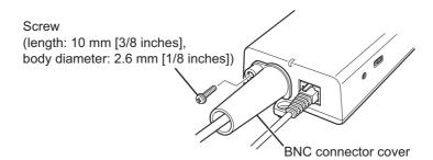
**4.** First pass the coaxial cable through the included BNC connector cover, then connect the coaxial cable to the BNC connector of the center adaptor.
