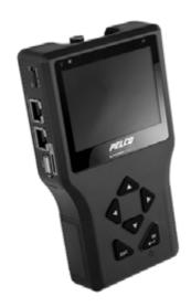
The **IPCT01** IP camera installation tool is a portable, battery-powered tool that provides flexibility in field installation of network video cameras with built-in Power over Ethernet (PoE) support. It connects directly to a camera to provide power, and display live video to adjust camera viewing angle and focus. Power can also be delivered through PoE bypass from an alternate power source. The tool offers a user-friendly, 3.5-inch touch screen for zooming and programming functions.
