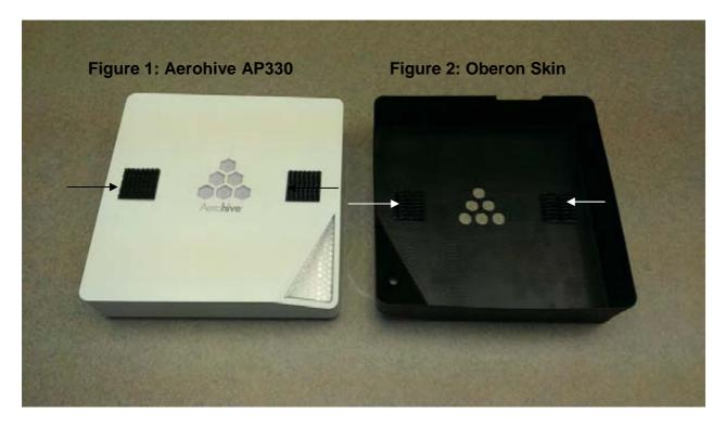
The following procedure should be used to install the Oberon skin on the Aerohive Networks AP330 access point.
