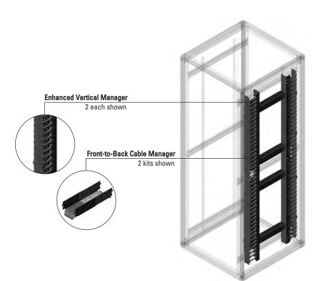
Enhanced Vertical and Front-to-Back Managers are accessories for the CPI M-Series MegaFrame<sup>®</sup> Cabinet System. MegaFrame Cabinet features integrated cable management space along both sides of the cabinet frame. Cable managers used within this space can be adjusted in depth (front-to-rear) to align cables with equipment.
