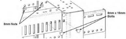
7. Install an 8 mm x 20 mm hex bolt and 8 mm star lock washer through the lower rail support and into one of the frame nuts on the lower frame bracket; this bolt should be in vertical alignment with the first upper bolt. <a href="Important: the star">Important: the star</a> washer must be used to ensure electrical bonding of the rail to the frame. Install an 8 mm x 16 mm bolt and 8 mm nut as far as possible from the first bolt; this bolt should be in vertical alignment with the second upper bolt
