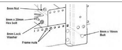
Set rail depth to final position and tighten all four bolts. Note: If rail is positioned with bolts at the end of the horizontal slots the rail depth will be set at depths of 25mm increments such as 400mm, 425mm, etc.
