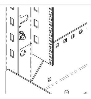
If you want the RMU numbering to start at the top: remove the rails, turn them over and mount on the opposite side of the frame. <u>Important: the star washers must be used to ensure electrical bonding of the rail to the frame.</u>
