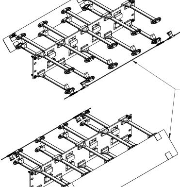
FRONT AND REAR PANEL SWINGS DOWN OR UP FOR CABLE ACCESS
