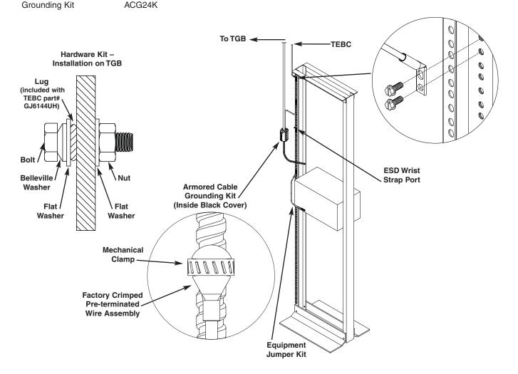
For the complete StructuredGround™ Grounding System offering, refer to www.panduit.com/dcgrounding.
