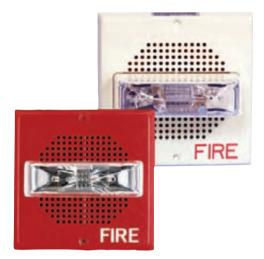
These Wheelock CH70 Multi-candela, Wall-mount Chime Strobes provide a low current draw, a choice of single-stroke or vibrating operation, an adjustable sound level, a chime tone adjustable from 800 Hz to 1200 Hz, and a choice of four light output intensities (15 cd, 30 cd, 75 cd, or 110 cd) in one unit. The strobes can be synchronized using SM (single) or DSM (dual) modules. They also have an attached mounting plate for easy indoor installation on a variety of electrical boxes.
