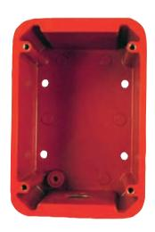
A red cast-metal weatherproof back box measuring 4.75 in. x 3.25 in. x 2.25 in. (12 cm x 8.3 cm x 5.7 cm) with ½ inch (12.7 mm) knockouts in the short sides. The back box is UL listed under UL38 and is UL certified for use in Canada. It has a NEMA rating of 3R and an environmental protection category of IP54.
