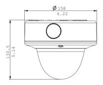
Dimensions in mm (in.) for surface mounting
