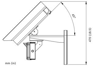
Camera housing tilted to maximum elevation.
