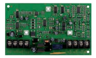
This module provides supervision of the battery lead connection in a system controlled by a Bosch Security Systems, Inc. 12 VDC control panel. This module may be used with other panels when referenced in the panel's installation/operation instructions. The module meets NFPA 72 requirements for battery lead supervision for fire alarm control panels (FACPs).
