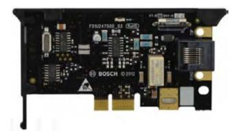
The B430 provides communication over the PSTN (Public Switched Telephone Network) by connecting the PSTN to the control panel. The module provides a single telephone jack, and easily installs into the control panel's on-board plug-in module connector.
