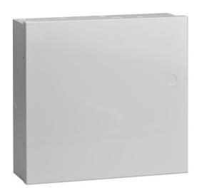
The B11 Small Control Panel Enclosure houses many Bosch control panels and modules. The enclosures are compatible with an enclosure tamper switch (D110 or ICP-EZTS), lock and key set (D101), and can hold one battery (up to 7 Ah).
