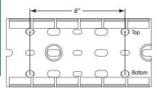
Minimum mounting rivet distance for ducts greater than  $2 \ensuremath{\,^{\prime}\!\!\!/}_{2}$  wide. Installed top and bottom.
