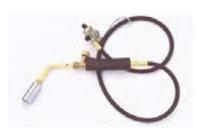
Light, portable propane torch for installing low-voltage products and smaller, conductor-sized, high-voltage (up to 15 kV) accessories. Includes hose, handle assembly, and regulator for disposable propane cylinder. Operates from disposable 14.1 oz. propane cylinders. Output: Approximately 20,000 BTU/hour. Handle and torch head not available separately. Regulator and hose assembly is product AD-3015-04.
