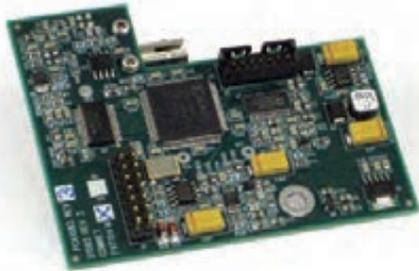
The ComNet™ FVT1031(M,S)1-P series video transmitter along with the ComNet™ FVR1031 series receiver supports simultaneous broadcast-quality video transmission of 10-bit digitally encoded video and return RS422 or Extended Distance Coaxitron data over one multimode or single mode optical fiber. The unit is designed to plug directly into the Pelco SpectraDome series, connecting power, video input and data via the Pelco electrical connector.
