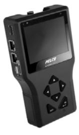
The **IPCT01** IP camera installation tool is a portable, battery-powered tool that provides flexibility in field installation of network video cameras with built-in Power over Ethernet (PoE) support. It connects directly to a camera to provide power, and display live video to adjust camera viewing angles and focus. Power can also be delivered through PoE bypass from an alternate power source. The tool offers a user-friendly, 3.5-inch touch screen for zooming and programming functions.
