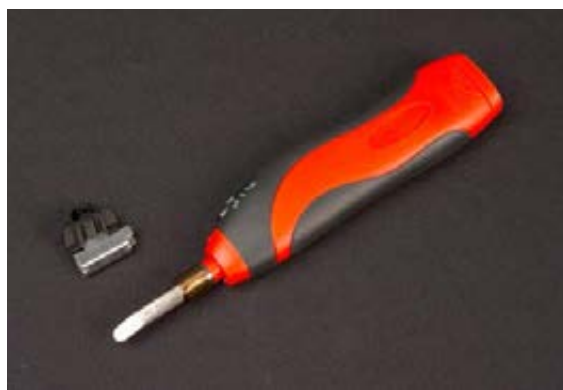
Handheld tool with installed tip and spring clip (bottom), and sleeve with finger protector (top)
