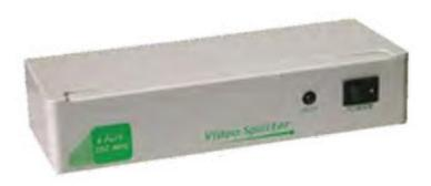
The Comprehensive low cost High Resolution Distribution Amplifiers support VGA, SVGA, XGA and multi sync monitors, with a transmission range of up to 50 meters. These distribution amps support a 350Mhz bandwith and are daisy chainable. The resolution on these units go up to 2300 x 1900 for maximum clarity.
