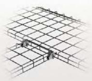
No sidewall cutting at intersections.
