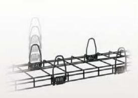
Optional snap-on sidewalls require no hardware or tools for installation. The sidewalls are available in three heights: 2" (50mm), 4" (102mm), and 6" (152mm).
