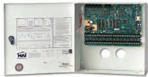
20A00-2 OmniPro II with enclosure
