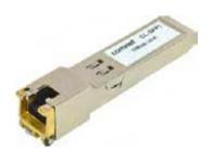
The ComNet™ CopperLine® CL-SFP is a small form-factor pluggable Ethernet extender module that improves bandwidth and distance of existing copper networks. It helps avoid installation costs of new fiber lines on site by allowing full 100Mbps Ethernet bandwidth to be extended over 2-wire twisted pair or coaxial cable.
