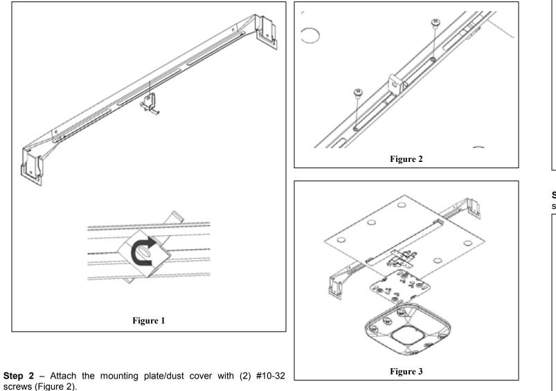
**Step 3** – Use the manufacturers T-Bar mount clip to attach the access point to the T-Bar Section on the mounting plate. An additional mounting plate provided by the manufacturer of the access point may be needed to attach the access point (Figure 3). Data cable(s) may need to be plugged in to the access point prior to attaching to the mount. Cisco access points use Cisco AIR-AP-BRACKET-2 for 2600/3600 series access points and AIR-AP-BRACKET-1 for 1140/3500 series.
