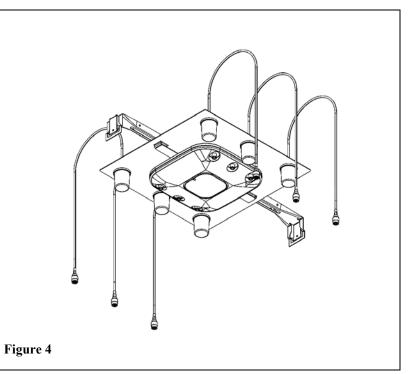
The assembled unit is now ready to be mounted above the ceiling tile.
