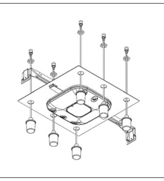
**Step 5** – Attach the hanger bar extensions to the hanger bar on both ends as shown in Figure 5. The hanger bar extensions should snap into place when installed correctly.
