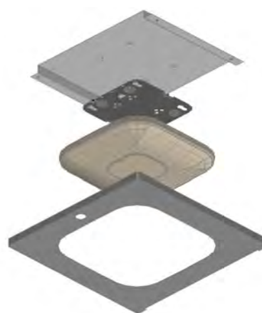
1) Model 1052-CCOAP and Cisco 1142 AP (not included) 2) Exploded view of the door, access point, access point mounting bracket, and assembly mount bracket
