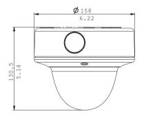
Dimensions in mm (in.) for surface mounting
