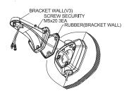
③ Insert the cable into the assembled mount, arrange the cable properly, fix it with screws and attach the mount onto the wall.
