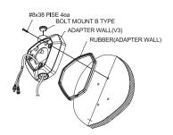
② Assemble the dome-camera installation mount and insert the cable into the mount
