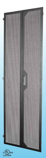
Split doors require a smaller swing clearance, allowing enclosure aisles to be placed closer together. ES enclosures that are 29" wide will only require a reduced door clearance of 14.25", with the 24" wide enclosures needing only 11.75".
