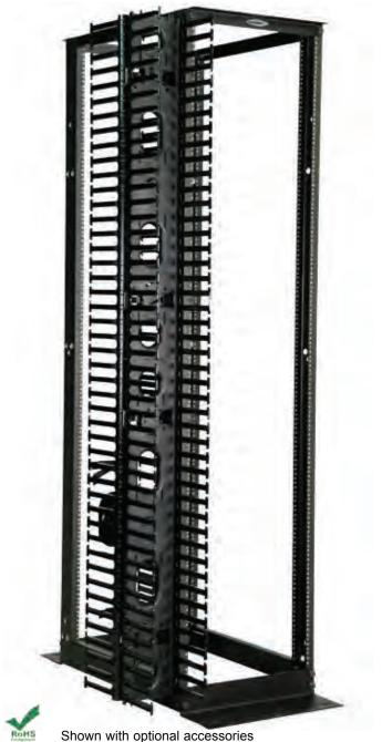
**DIMENSIONS:** 84"H x 20.6"W, Rail Depth Ranges from 24" to 36" RACK SPACES: 45 RMU · 19" EIA 310-D Compliant WEIGHT CAPACITY: 1500 lbs. when networked; 1000 lbs. free standing **CONSTRUCTION:** 12 Gauge Cold Rolled Steel and Extruded Aluminum SHIPPING WEIGHT: Please see Part No. Description
