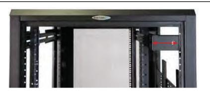
Great Lakes offset rail kit allows one set of rails (on either side of the enclosure) in 30"W ES enclosures to be shifted inward, creating 6" of space (from the outside of the rail to the inside edge of the enclosure). This 6" of space is ideal for routing high density cable bundles along one side of an enclosure; either independently or by using vertical cable troughs.
