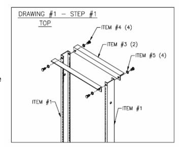
corresponding holes in vertical uprights. Formed leg of top angle should be facing toward you.
