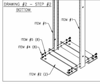
C. Turn vertical upright assembly over (rotate 180 degrees) and repeat steps A and B. Finger tighten only.
