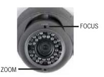
Insert rubber weatherproofing plugs (2x) firmly into the ZOOM and FOCUS screw-holes to ensure a weatherproof seal.
