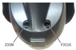
4. Insert rubber weatherproofing plugs (2x) firmly into the ZOOM and FOCUS screwholes to ensure a weatherproof seal.
