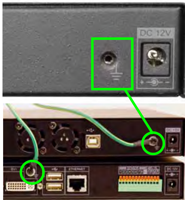
Figure 1.0 Connect the grounding cable from the expansion bay to the Blade.
