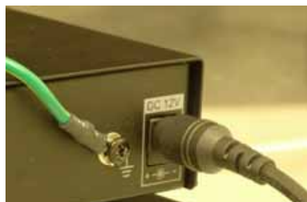
Figure 1.2 Connect the power cable
