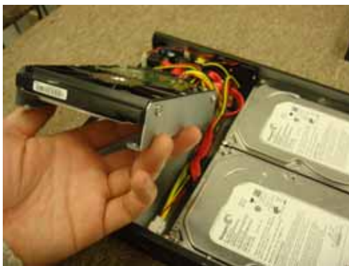
Figure 3.3 Lift the hard drive out of the bay, and carefully disconnect the SATA power and SATA data cable.
