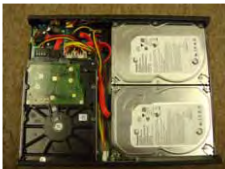
Figure 3.2 With the hard drive in place, flip the unit over with your hand clasping the hard drive so that it does not fall out. Tighten the four screws underneath the unit to secure hard drive.
