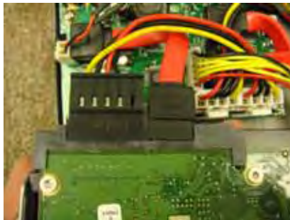
Figure 3.1 Connect the SATA power cable and SATA data cable. Make sure connections are in all the way.
