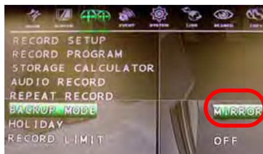
Figure 2.5 Record setup menu. Select MIRROR under BACKUP MODE.
