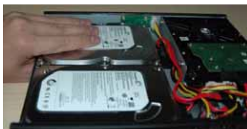
Figure 3.6 Clasp your hands on the hard drive and flip over.
