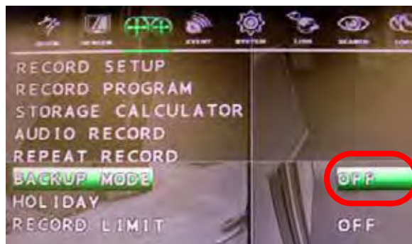
Figure 2.0 Record setup menu. Select OFF under BACKUP MODE.
