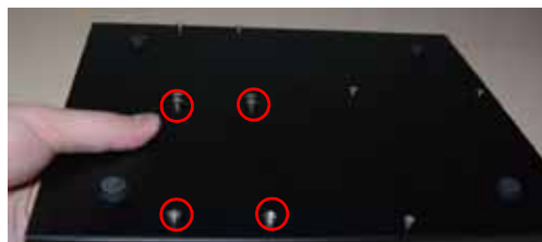
Figure 3.7 While holding the hard drive, screw in the four screws to secure the hard drive in place.
