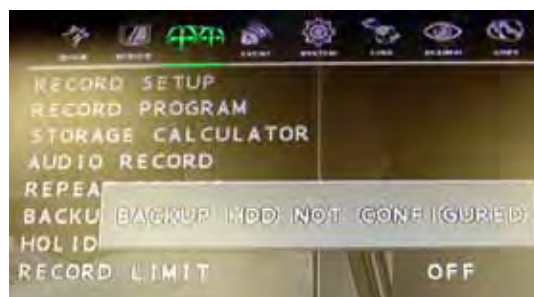
Figure 2.6 Error message during Recording configuration. Double-check and make sure that you correctly set the HDD CONFIGURATION menu. The hard drives must be set to BACKUP mode.
