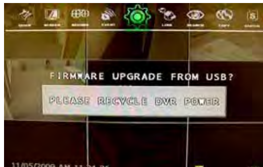
Figure 1.6 Power off the Blade for several seconds and power back on after the prompt appears.
