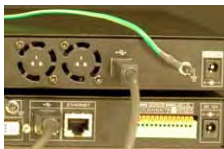
Figure 1.1 Connect the USB cable to the Blade and expansion bay.
