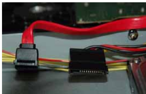
Figure 3.8 SATA connectors. Data connector shown on the left; power connector on the right.
