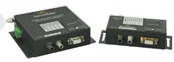
Dymec models 5843 and 5844 are hardened fiber optic Link/Repeaters that convert RS232 or TTL level copper to amplitude based fiber output. Supports data rates from dc to 250k bps, DCE or DTE port configuration and a diagnostic/test mode that allows testing of the copper and fiber connections before the connected IED is active in the network.
