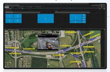
Designed for large surveillance installations, XProtect® Smart Wall is an advanced video wall for control rooms and alarm centers. It enables operators to obtain an optimal situational overview and coordinate response activities.
