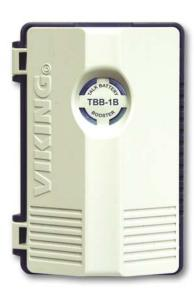
The **TBB-1B** will boost talk battery voltage up to 48VDC, and current up to 26mA on single analog line extensions behind PABX's and electronic key systems. This is helpful for powering line powered devices such as touch tone dialers and emergency phones on low voltage and/or low loop current extensions.
