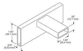
Note: .065" (1.65 mm) thick tubular stringer. Combined area of both stringers is a minimum of .40 square inches (260 square millimeters)
