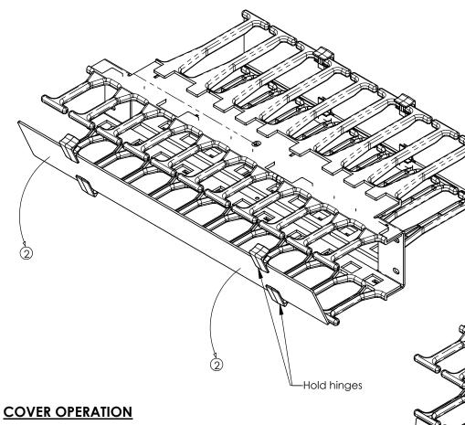
To gain access to the cables within the panel, the cover can be hinged open from the top or bottom, or it can be completely removed.
