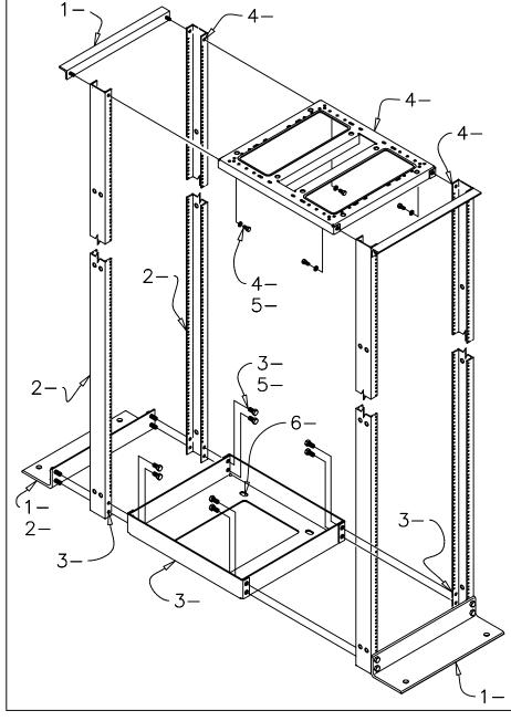
The new ExpandaRack Extension Kit is designed to easily convert one CPI Rack Assembly into a high capacity 4—Post Frame.
