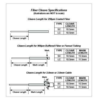
\*Alternative cleavers were also tested. Those with a quaranteed maximum 1° cleave angle for single-mode fibers and a maximum 2° cleave angle for multimode fibers provided acceptable results.
