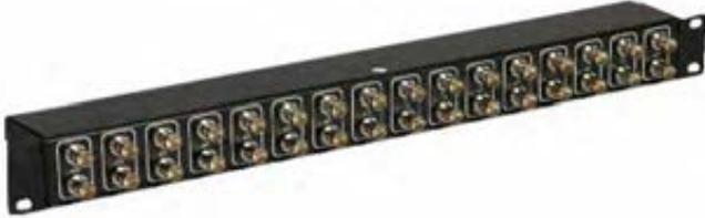
The **RM-CX06-16R** is a 19" rackmount, 16 channel, surge protector ideal for protecting expensive video equipment such as multiplexers from damaging transients coming from exposed video lines. This device utilizes a three-stage hybrid topology to clamp over-voltage transients and mitigate damaging sneak currents.
