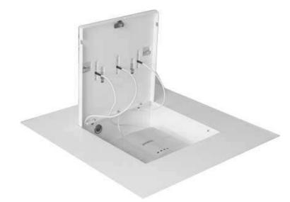
Step 2 – (**Enterasys Hipath APs Only**) Install the access point so that the three antenna connectors are facing away the door lock. Securely fasten the *access point's mounting plate* to the mounting holes on the back wall of the enclosure using (4) # 8-32 screws. Attach the screws to the *outer* hole pattern. Attach the *Access Point* to the mounting plate. Proceed to *Step 3*.
