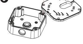
**5.** Reattach the cable plate to the cover, ensuring that the rubber seal is in the correct position.
