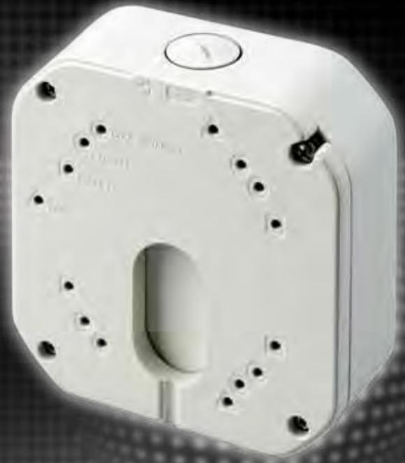
The versatile MNTV2XB Junction Box Mount is compatible with select Pinnacle & SyncroIP Dome Cameras, Bullet Cameras, plus Wall/Ceiling Mounts (refer to features/specs for more details). The Junction Box provides a concealed area for cable management in addition to provision for conduits with dual side & single rear conduit entries. MNTV2XB is suitable for indoor or outdoor use with an IP66 rating.
